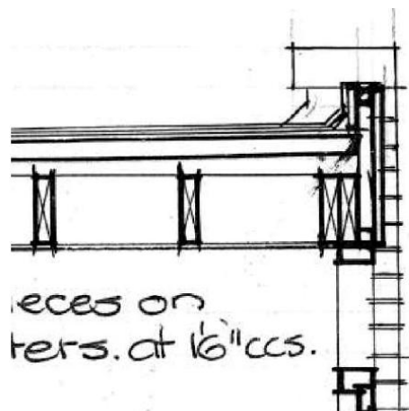
Figure 8: Sectional roof structure detail produced by the original project architect
