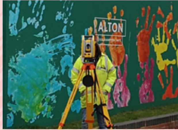
Surveyor capturing the CCTV and Utilities survey data using the Trimble Theodolite.
