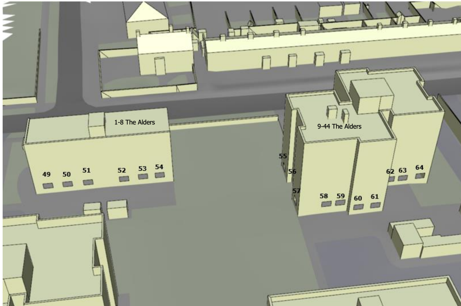
Figure 4 Window Locations Assessed – Existing Surrounding – 1-44 The Alders
