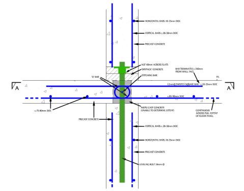
Fig 3.4: section of connection between adjacent floor panels (from GBG report)
