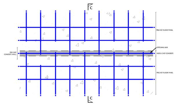
Fig 3.3: plan of connection between adjacent floor panels (from GBG report)
