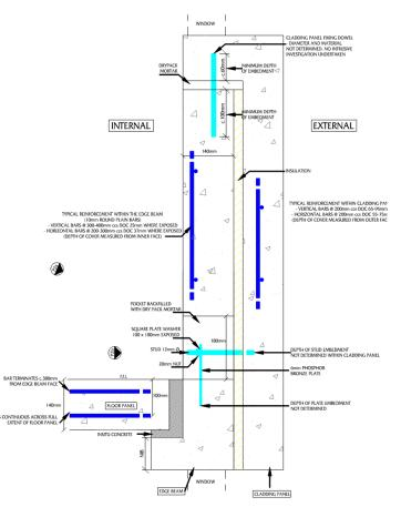
Fig 3.2: connection of façade panel to edge beam (from GBG report)
