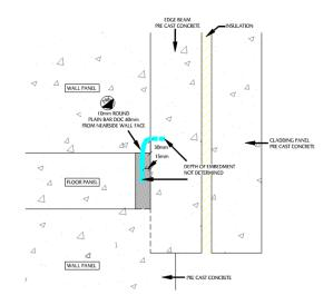
Fig 3.3: connection details of edge beams to wall supports (from GBG report)
