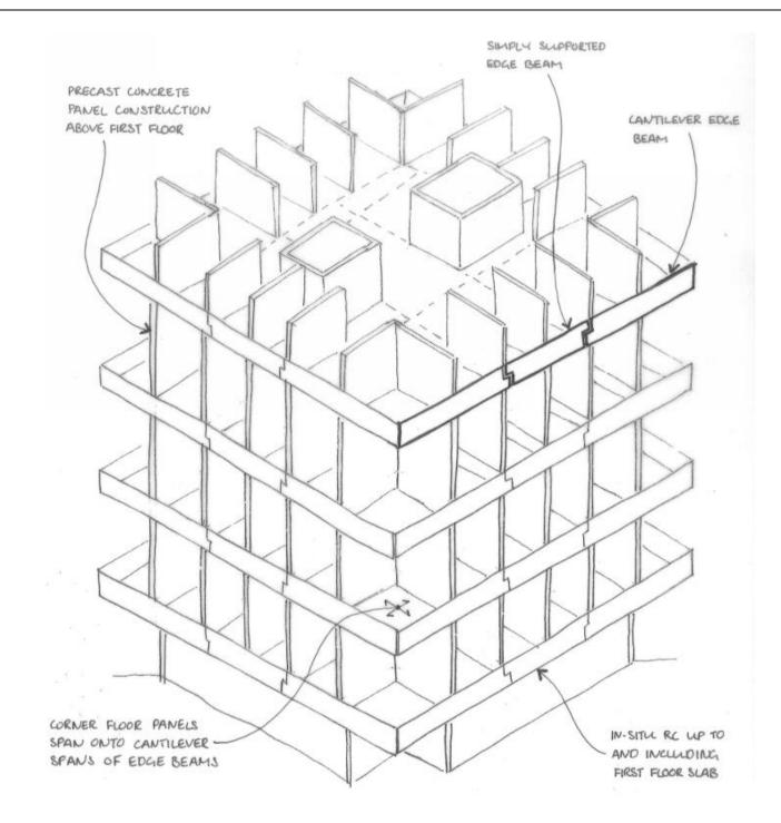
Figure 1.1: Isometric showing the existing structure of the towers
