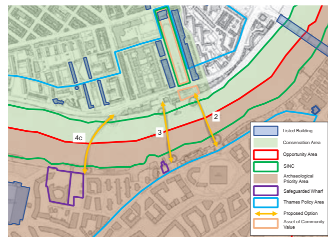
Planning constraints plan illustrating significant site designation applicable to the identified potential landing options
