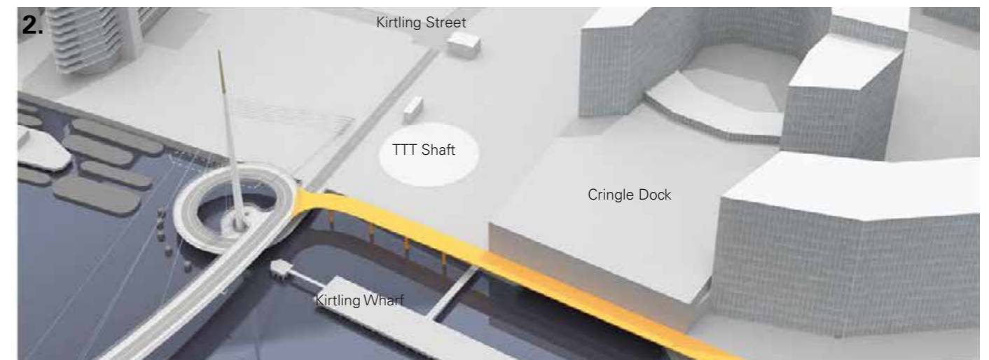
Location 4C concept arrangement with a connection to a High Level Walkway over Cringle Dock and Kirtling Wharf, at the top of the deck spiral.
