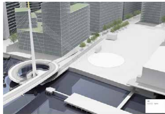
Visualisation of concept design landing arrangements for Location 4C (north landing above and south below)
