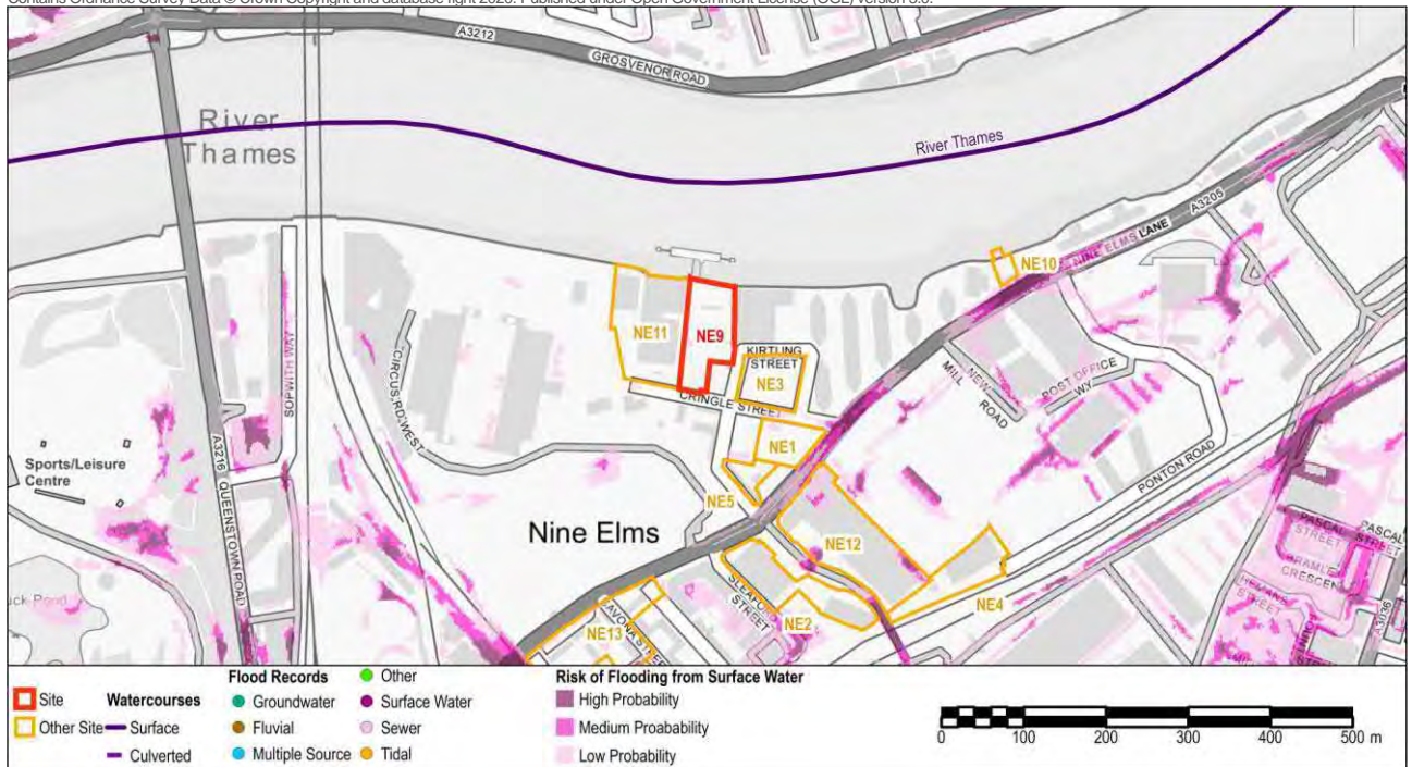
Figure D - Risk of Flooding from Surface Water (RoFSW)
