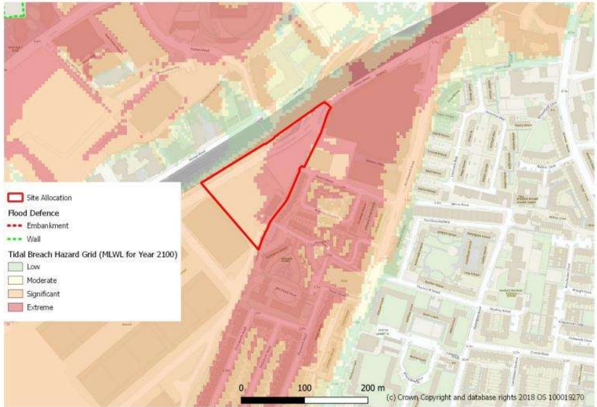
New Covent Garden Market Apex Site - London Thames Breach Assessment - Maximum Flood Hazard (2100)
