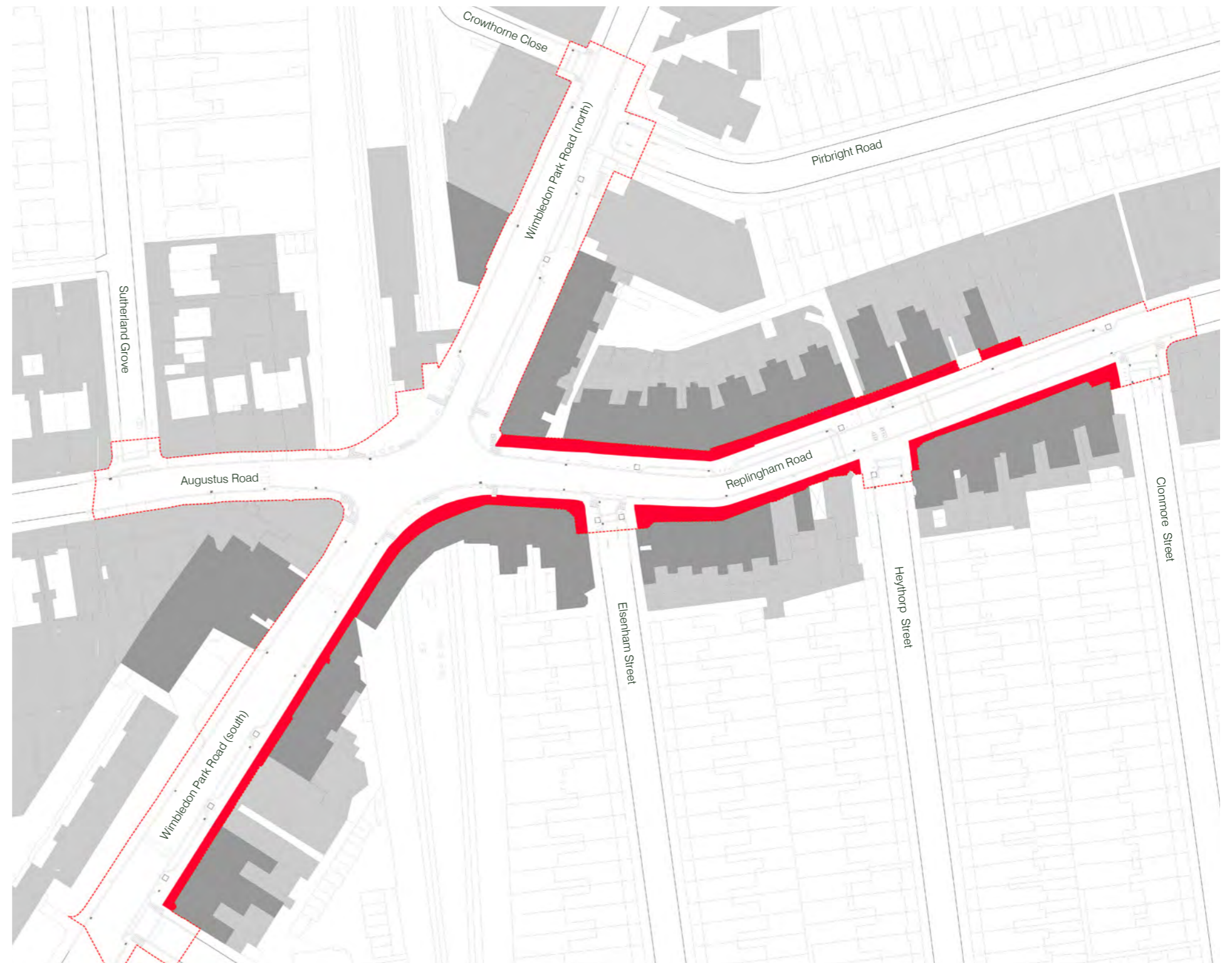
Figure 15. Paving treatment beyond highway boundary
