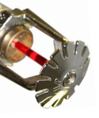
The individual sprinkler heads in a room with a fire will only activate when the room temperature exceeds the pre-set temperature of the sprinkler head - normally between 57 to 68 degrees centigrade. The heads operate as individual heat sensors - water is only released in the area where there is a fire. Evidence suggests that the chances of a sprinkler malfunctioning are extremely remote - estimates put this at worst 1 in 5 million and at best 1 in 16 million.
