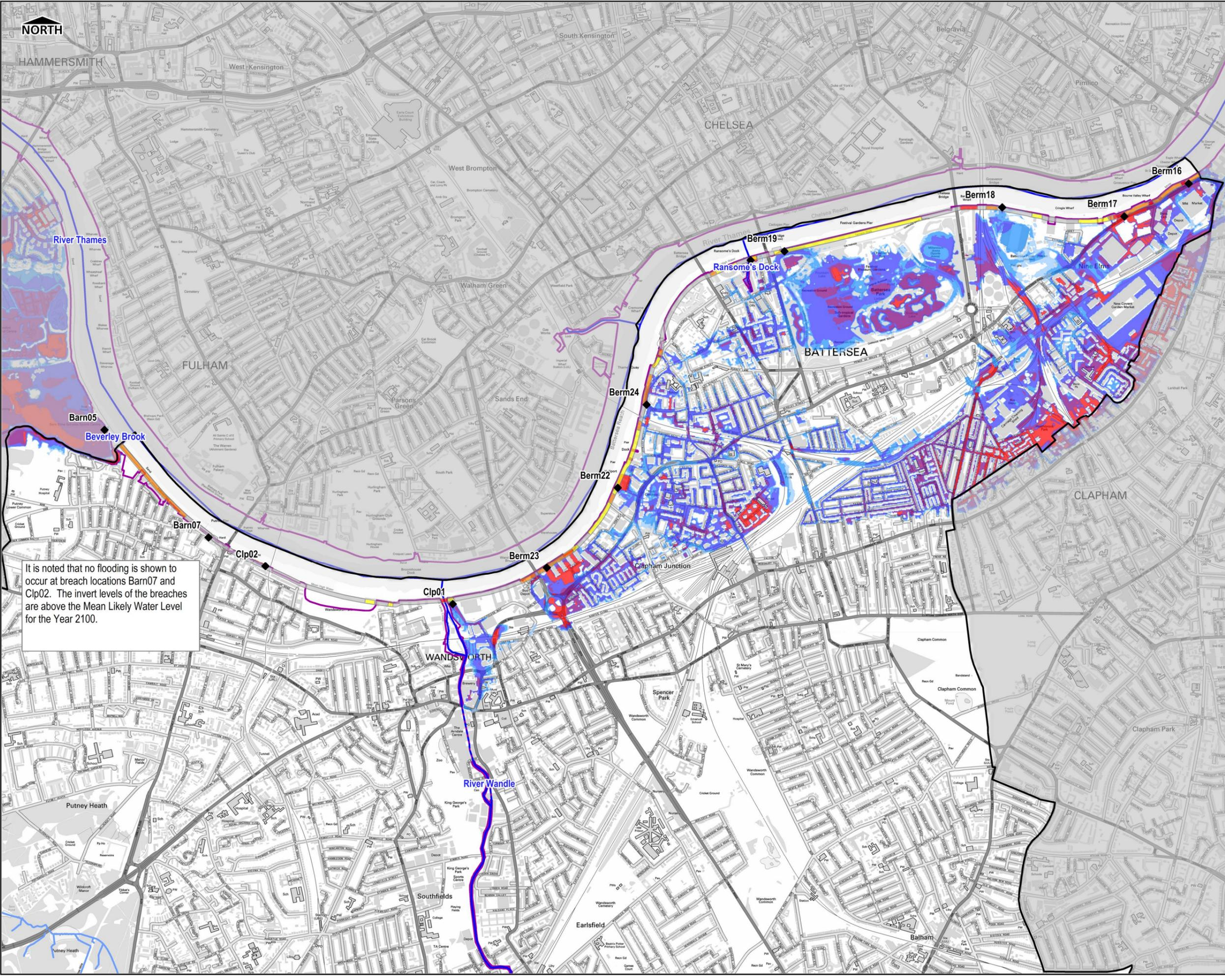
It is noted that no flooding is shown to occur at breach locations Barn07 and Clp02. The invert levels of the breaches are above the Mean Likely Water Level for the Year 2100.
